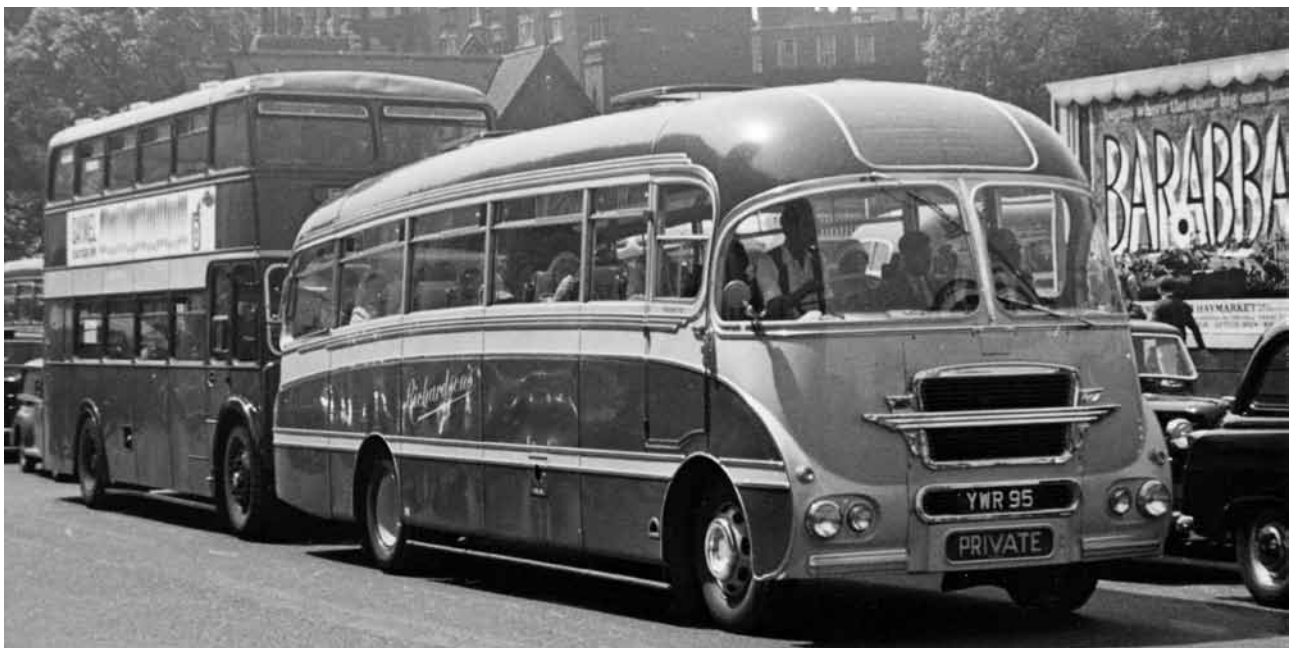
The version of the Burlingham Seagull body carried by YWR 95, a Ford 570E, was far less elegant than the original Seagull design of coachwork. This coach wore the green and cream livery in which it was purchased rather than the standard red and cream colours of Richardson's Coaches.
