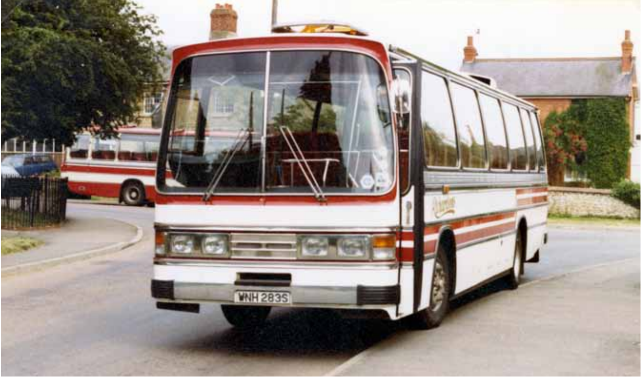
By 1977 when WNH 283S was new, the Duple Dominant II body was current and fitted to a Bedford YMT chassis for Richardson's.
