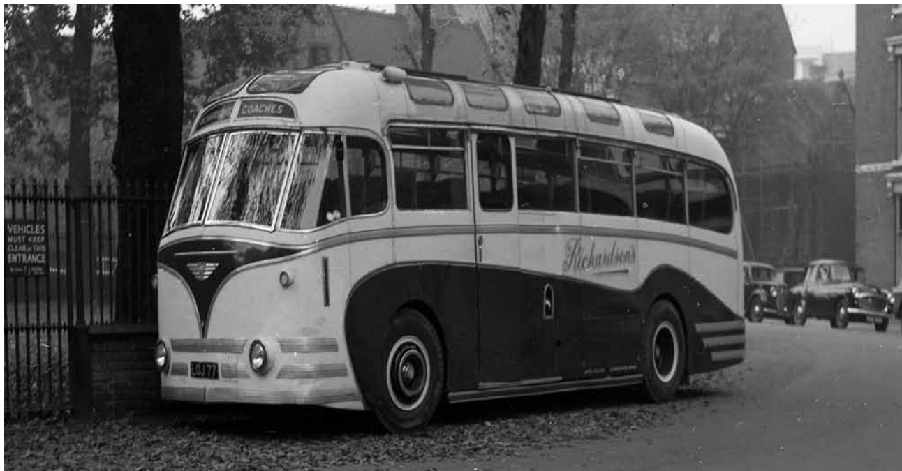
One of the two Bellhouse Hartwell bodied coaches in Richardson's fleet is shown here. Registered LOJ 77 it was an A.E.C. Regal IV and it seated thirty-seven passengers.
