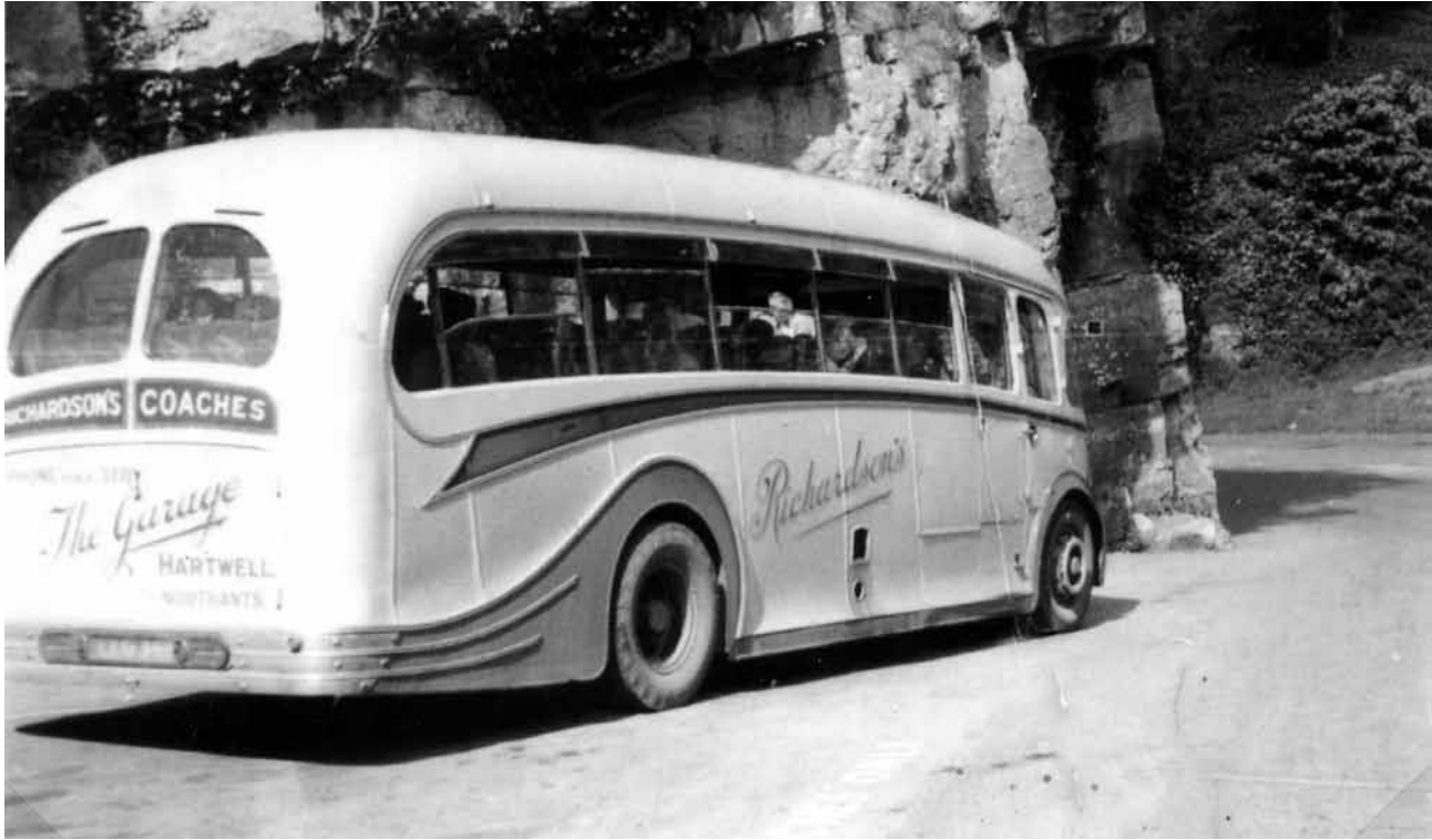
A rear view of LLG 368 which was a Leyland Titan TD3 that started life with Oldham Corporation as BU 8439 in 1935 as a double deck vehicle. It was rebodied with thirty-three seat Harrington coachwork shown in this picture in December 1948 when it was re-registered LLG 368.
