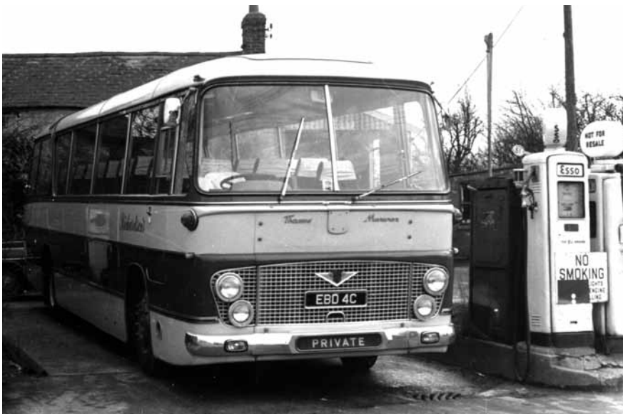
EBD 4C, the Duple Mariner bodied Ford 676E is illustrated here with its very useful fifty-two seating capacity. (Photo courtesy M R Knight).
