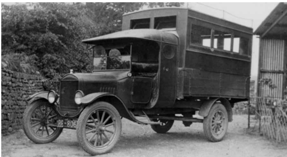
Ford T - RP 806 - photographed at Belgrove's Cold Higham premises on 12th August 1926, from which it can be seen that the machine was basically a lorry which could be converted for use as a passenger carrying vehicle.
