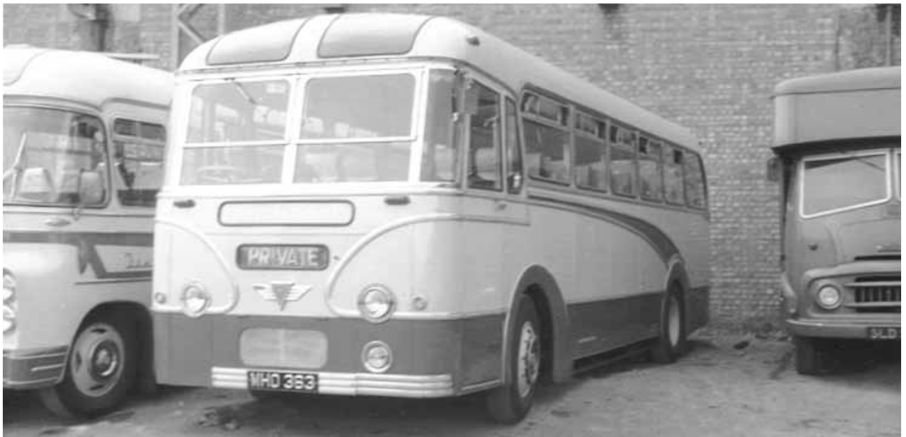
One of the two A.E.C. Reliances taken from Taylor's was MHO 363 having a Mann Egerton body seating forty-three passengers.
