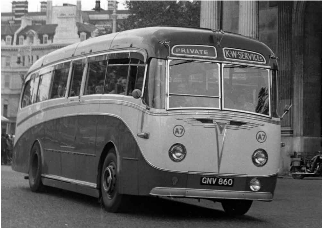
A.E.C. Regal IV GNV 860 with its fully-fronted Yeates body immediately made the rest of KW's coaching stock look dated. It was, therefore, the flagship of the fleet for two or three years. (Photo courtesy ATPH/Hustwitt)
