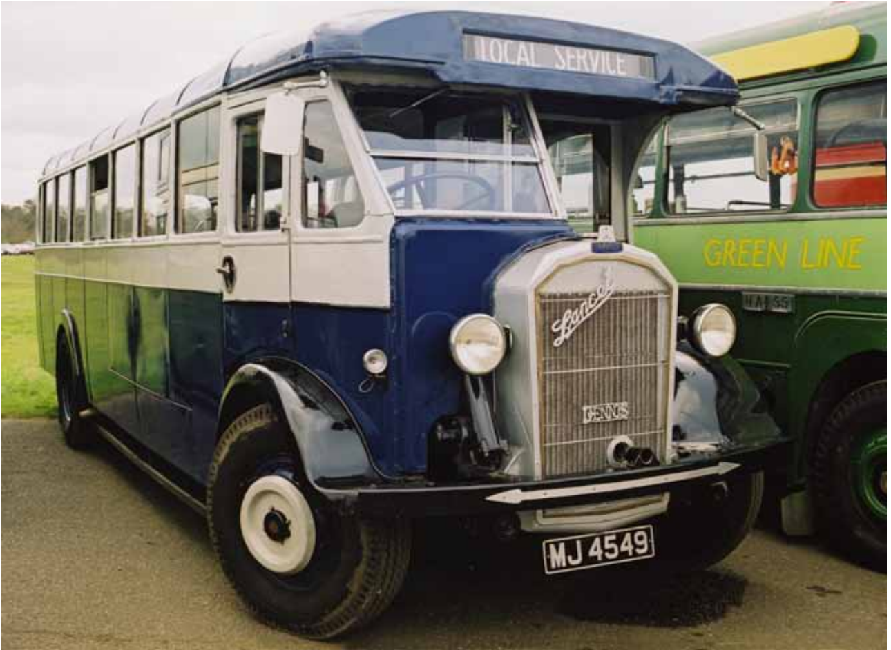
Fortunately the thirty-two seat Short bodied Dennis Lancet MJ 4549 has been preserved and is seen in this photograph at a rally at Brooklands.
