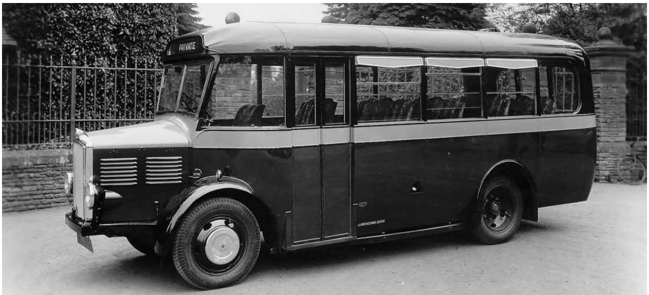
Equally fortunate is the survival of this picture of twenty-seat Grose bodied Dennis Ace MJ 4550 as supplied new to G I Smith of Westoning in June 1934.
