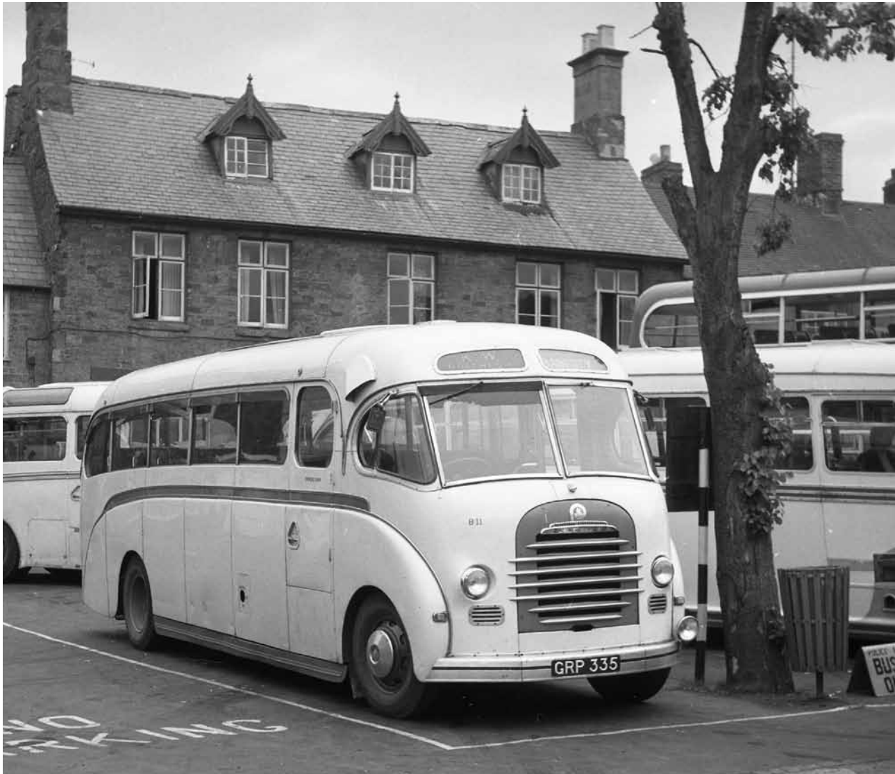
GRP 335 was a Bedford SB with Duple Vega coachwork and it was photographed at Banbury having worked one of KW's stage-carriage routes into this Oxfordshire market town. (Photo courtesy R Marshall)
