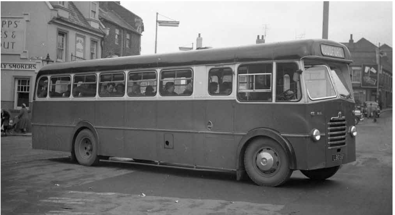
This time an offside view of a Duple Midland bodied Bedford SBG. Again photographed at the Mayorhold, Northampton this illustration shows LBD 512 working local stage-carriages services. (Photo courtesy R Marshall)
