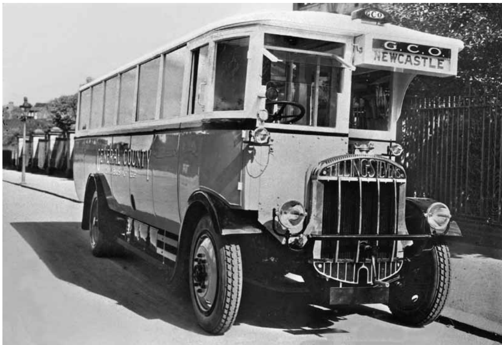
UP 218 was probably bought second-hand to replace the burnt out Lancia RP 5477. It was a Tilling-Stevens B10 that is seen here in the livery of General County Omnibus Co Ltd, Newcastle prior to registration.
