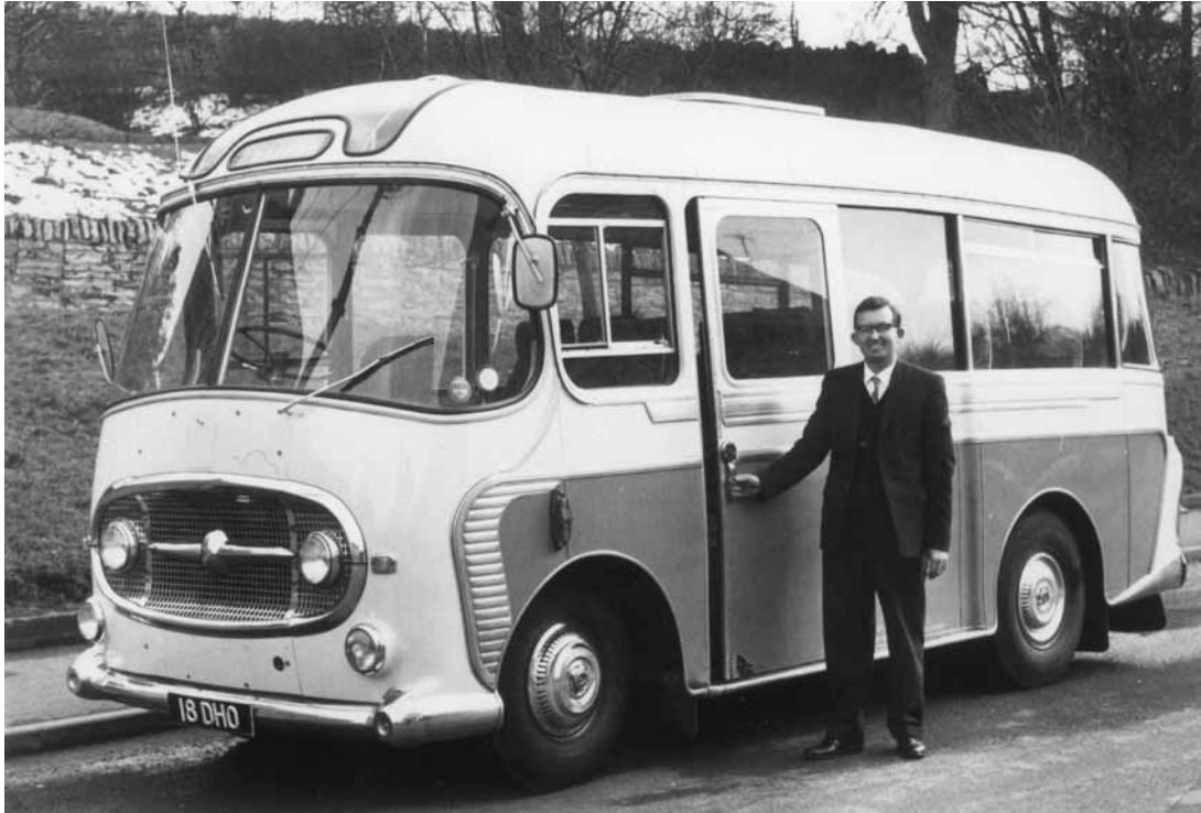
Pete Skinner stands alongside 18 DHO which comprised a Bedford J2 chassis mounted with a Plaxton Consort III eighteen-seat body, about to leave for a private hire trip to London.
