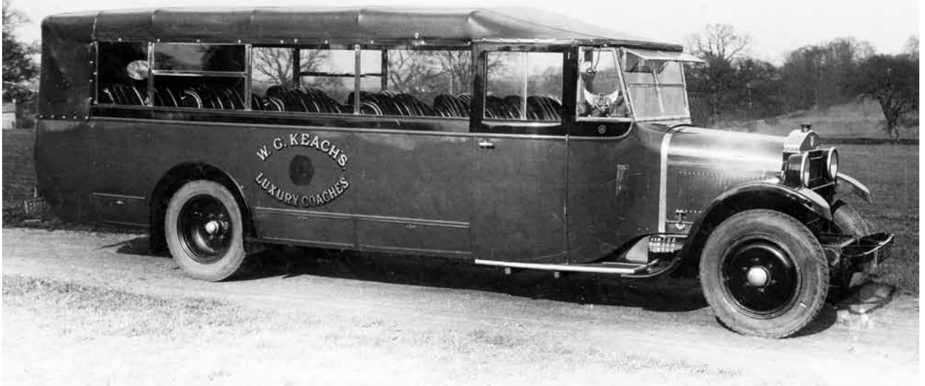
A great view of Walter Keach's REO registered RP 3829 fitted with a twenty-seat all-weather body.
