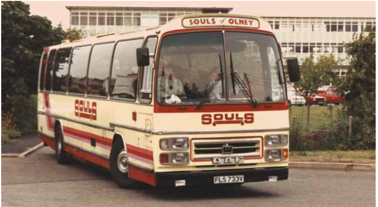
Seen leaving Roade School in FLS 733V, a DAF MB200 fitted with a fifty-seven seat Plaxton Supreme IV body.
