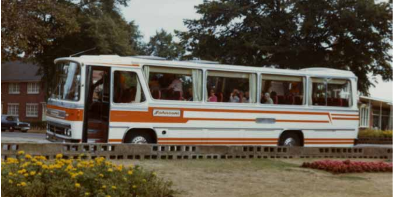
Either HRP 436 or 7N is the subject of this photograph and shows a Caetano Estoril II bodied Bedford YRT. Apparently these coaches were extremely sluggish due to the weight of the Caetano bodywork.
