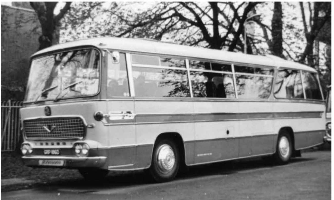
GRP 186D was one of a pair of Bedford VAM 14s fitted with Duple Bella Venture bodies seating forty-five passengers when new in February 1966.
