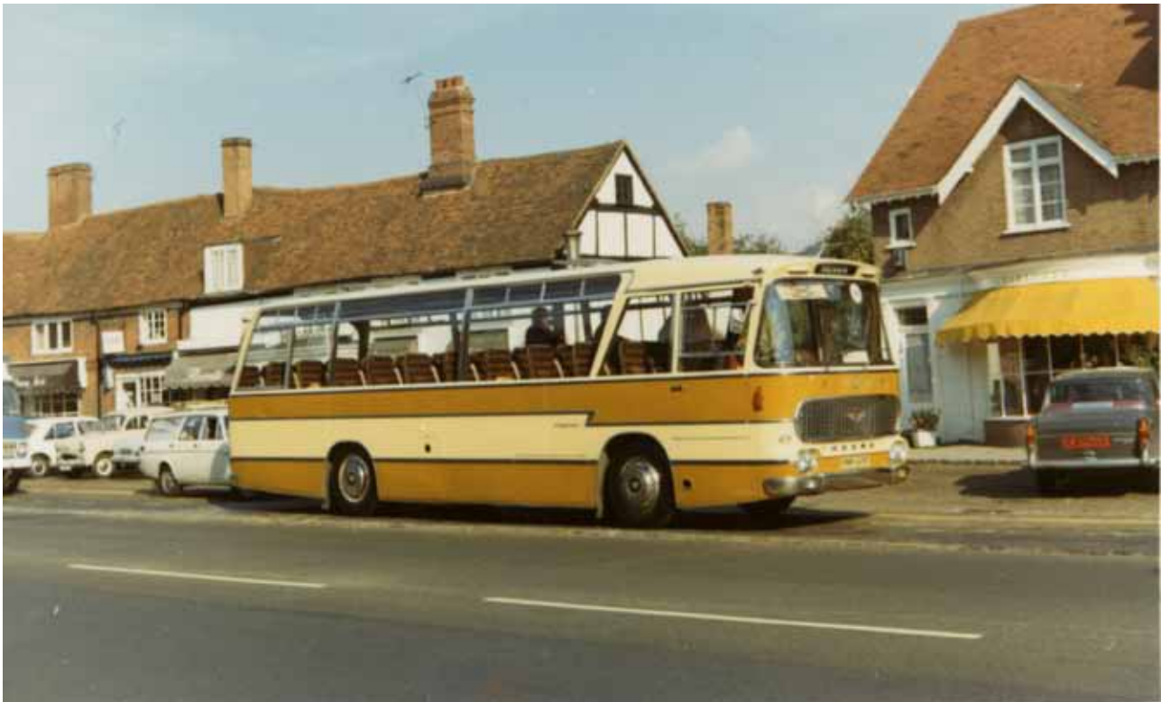
ONR 685F was a Ford R192 with Duple Viceroy forty-five seat bodywork which was just two years old when Johnson's bought it in July 1970.
