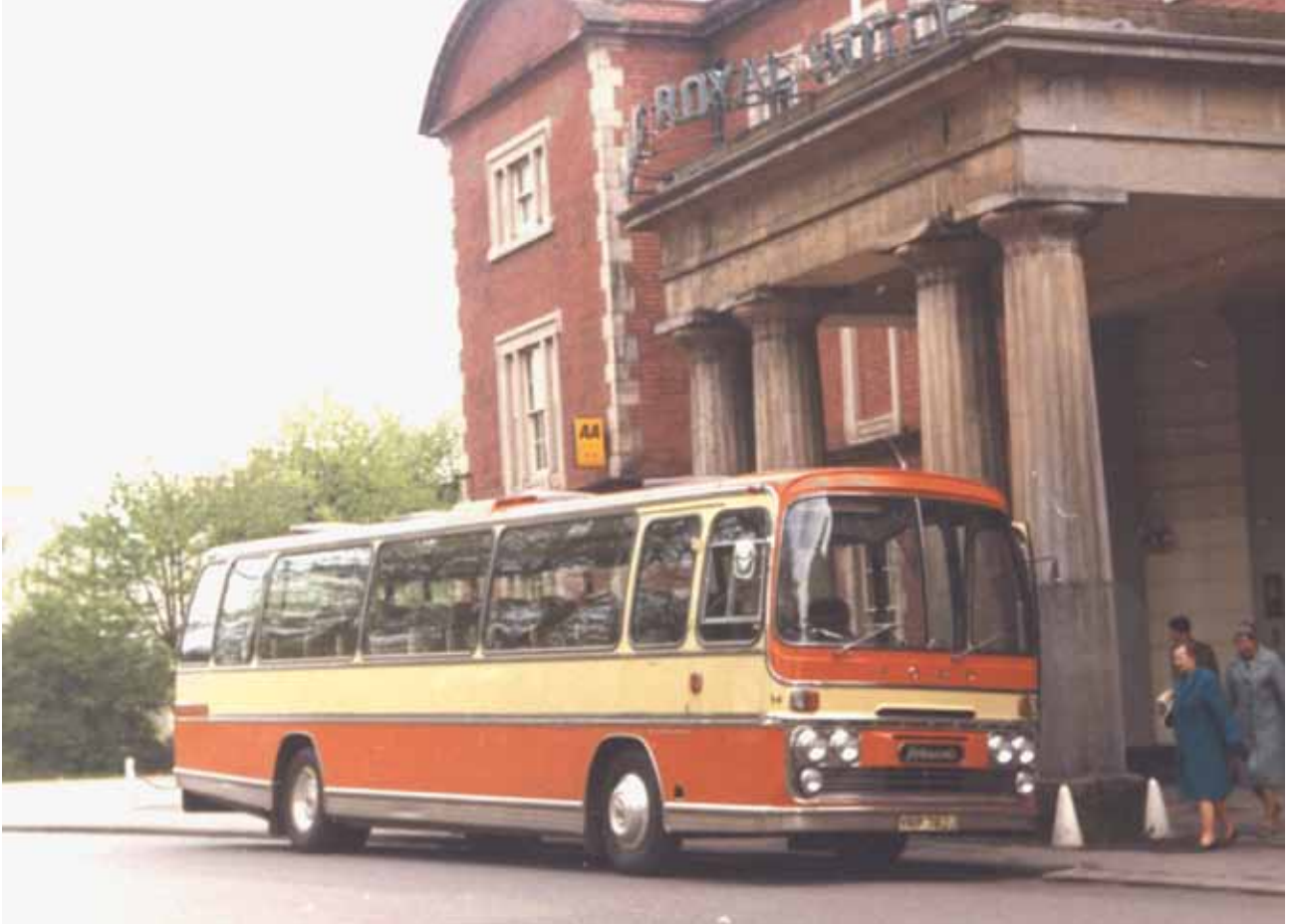
Plaxton Panorama Elite II bodied Ford R226 carrying the registration YRP 782J was a long way from home when photographed at Ashby-de-la-Zouch.
