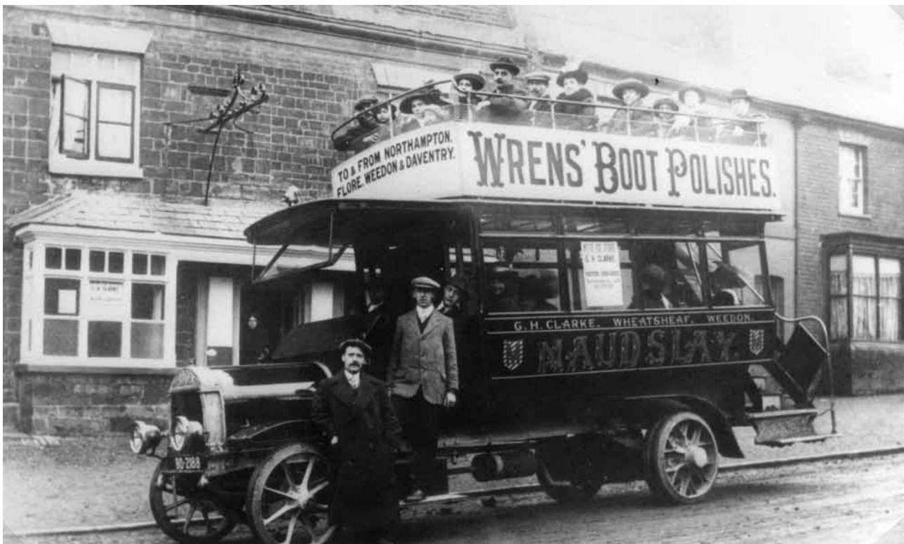
Ex-Maudslay demonstrator BD 2188 stands outside the Wheatsheaf at Weedon with a full compliment of passengers when the vehicle was new in 1914. This bus was equipped with a folding windscreen and an illuminated destination display, both features which were unusual as early as 1914.
