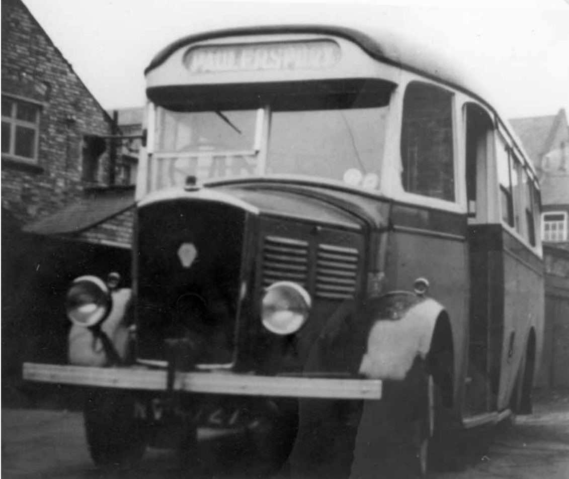
Lenny Edward's Dennis Ace registered NV 4727 is seen here in the yard of the Plough Hotel, Northampton. It had a twenty-seater Willowbrook body.
