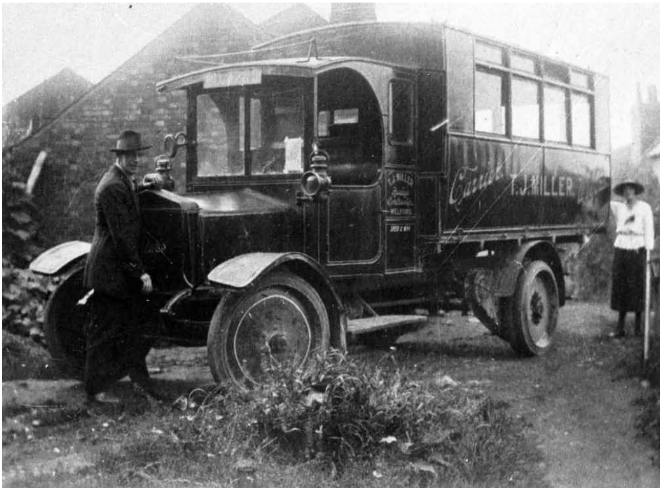
This photograph illustrates Thomas Miller's chain-driven Alldays & Onions twelve-seater lorry-bus registered BD 4783.
