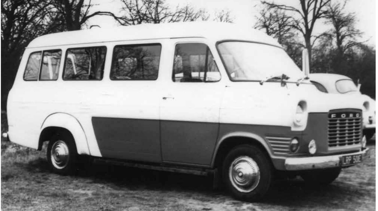
Purchased to replace 727 DBD was LRP 50E, a Ford Transit with twelve seat Williams Deansgate body. Not a particularly attractive vehicle although very useful.
