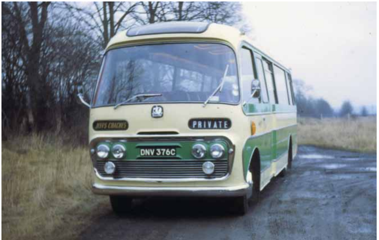
In the Author's opinion the Plaxton Embassy IV body was an elegant design and looked well on DNV 376C, a 1965 Bedford SB5. The Helmdon Depot provides the setting for this photograph.
