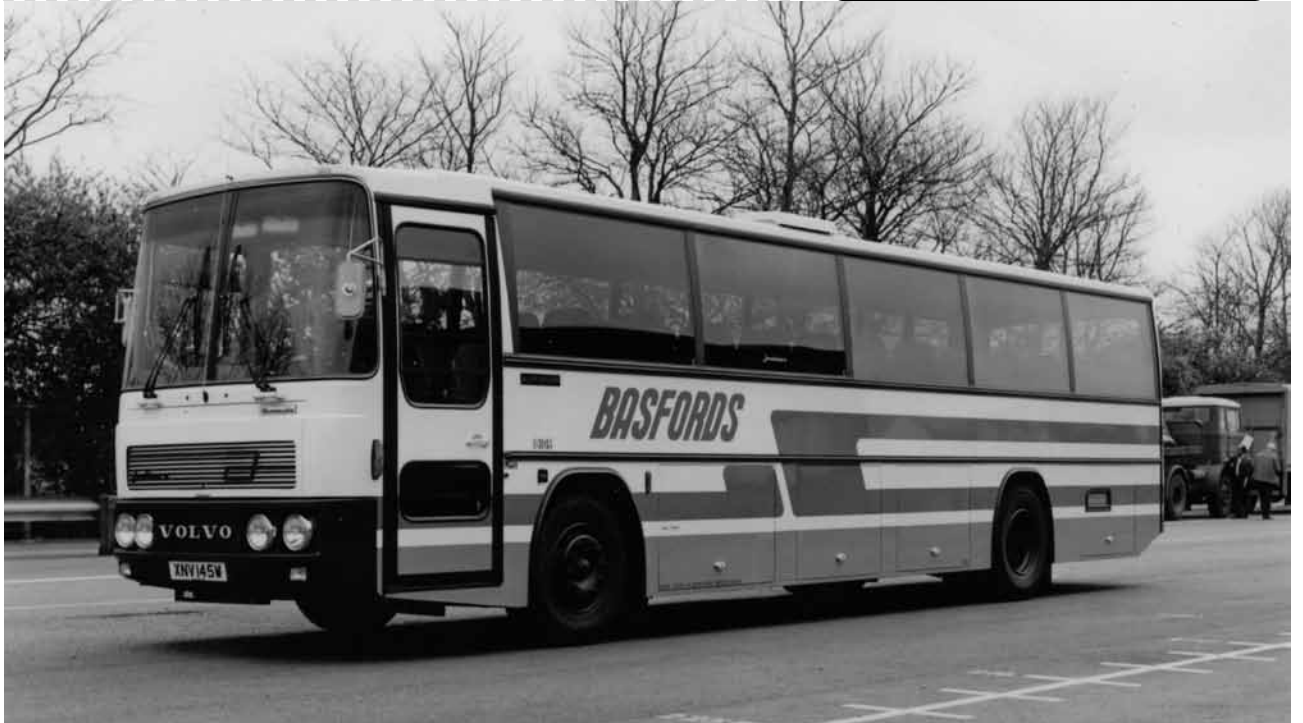
XNV 145W was a 1981 Volvo B10M-61 mounted with a fifty-three seat Jonckheere Bermuda body. Although very well appointed internally, the rather forbidding front end was probably not as pleasing as some of Jonckheere's later designs.
