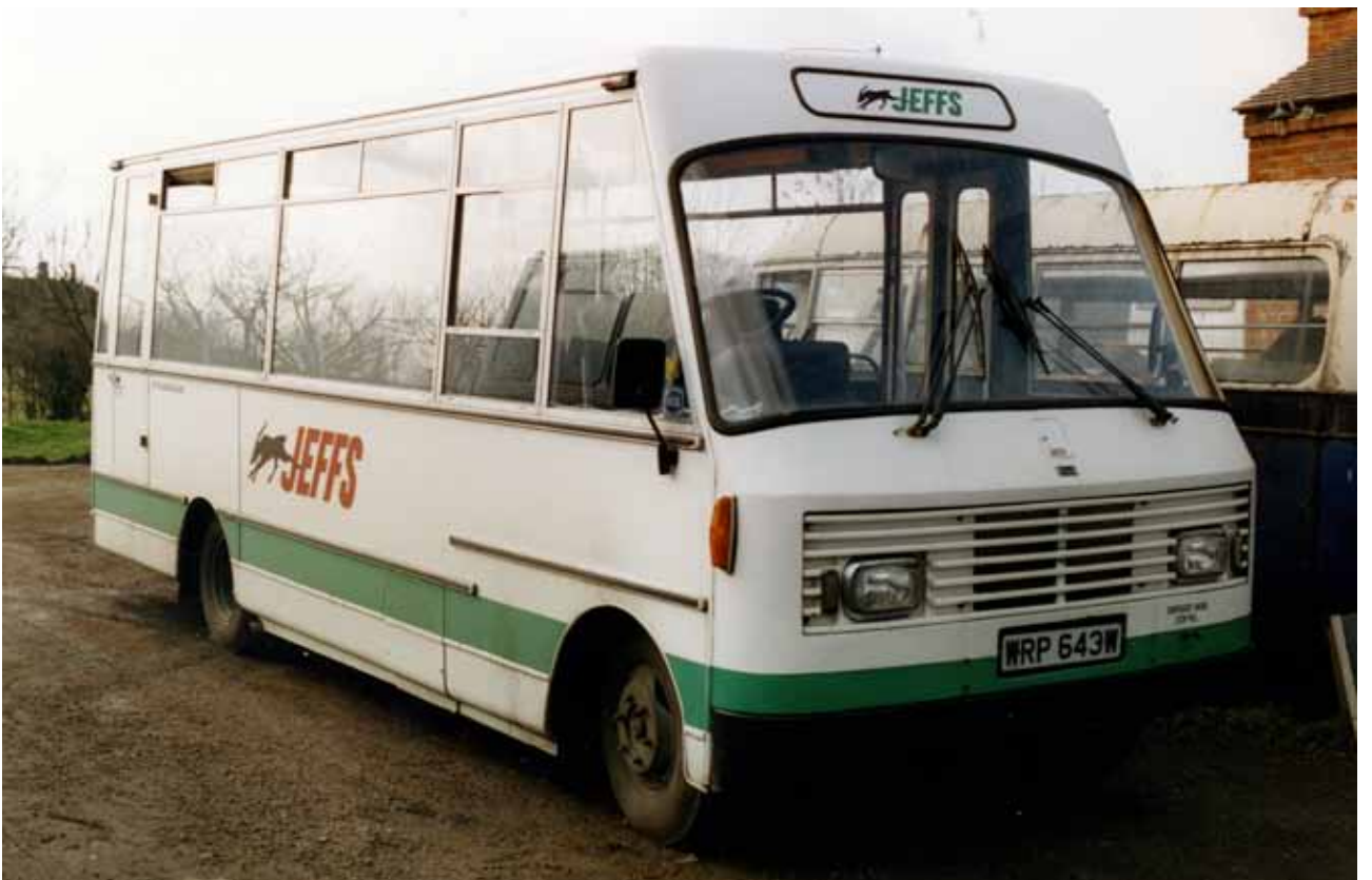
WRP 643W was a twenty-five seater Moseley Faro III bodied Ford A0609 some five years old when acquired from Payne's, but it continued in service for another eight years.
