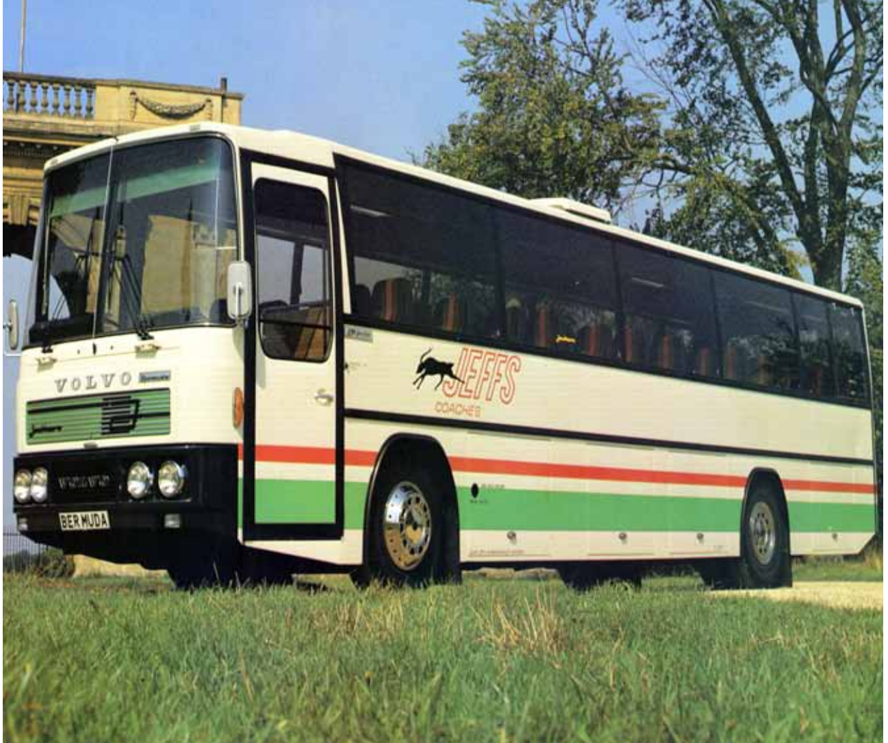
This handsome Jonckheere Bermuda bodied Volvo B58-61 was photographed prior to registration but it soon became PBD 776V, the first of many Jonckheere bodied coaches in the Jeffs' fleet. (Photo courtesy Volvo Bus (GB) Ltd)
