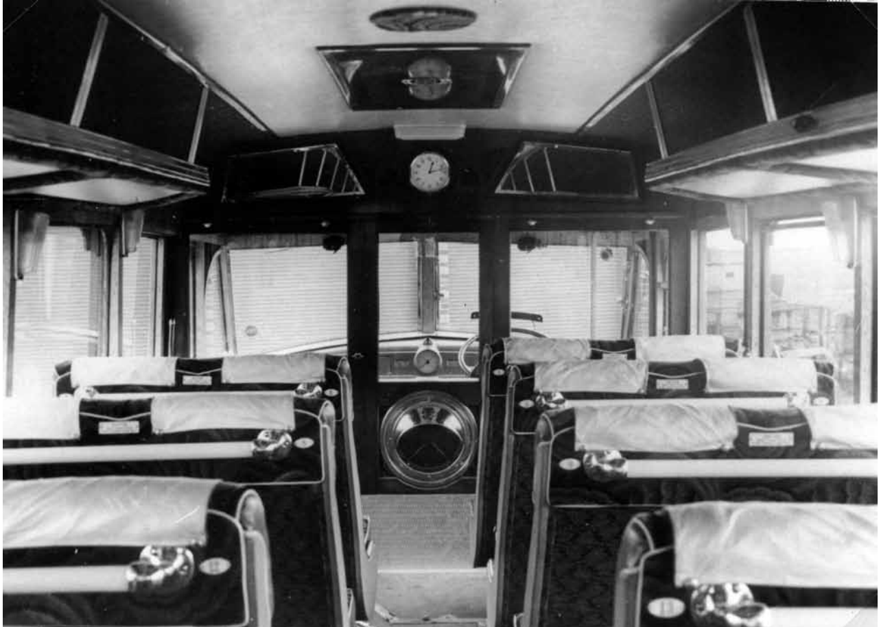
The sumptuous interior of the Thurgood body of JNM 735 complete with Clayton-Dewandre heater.
