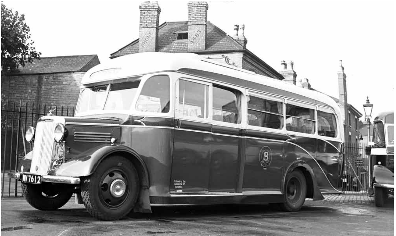
In this view Fred Buckby's modern looking Bedford WTB - NV 7612 - with its 25-seater Willowbrook body is depicted. (Photo: R Marshall collection)
