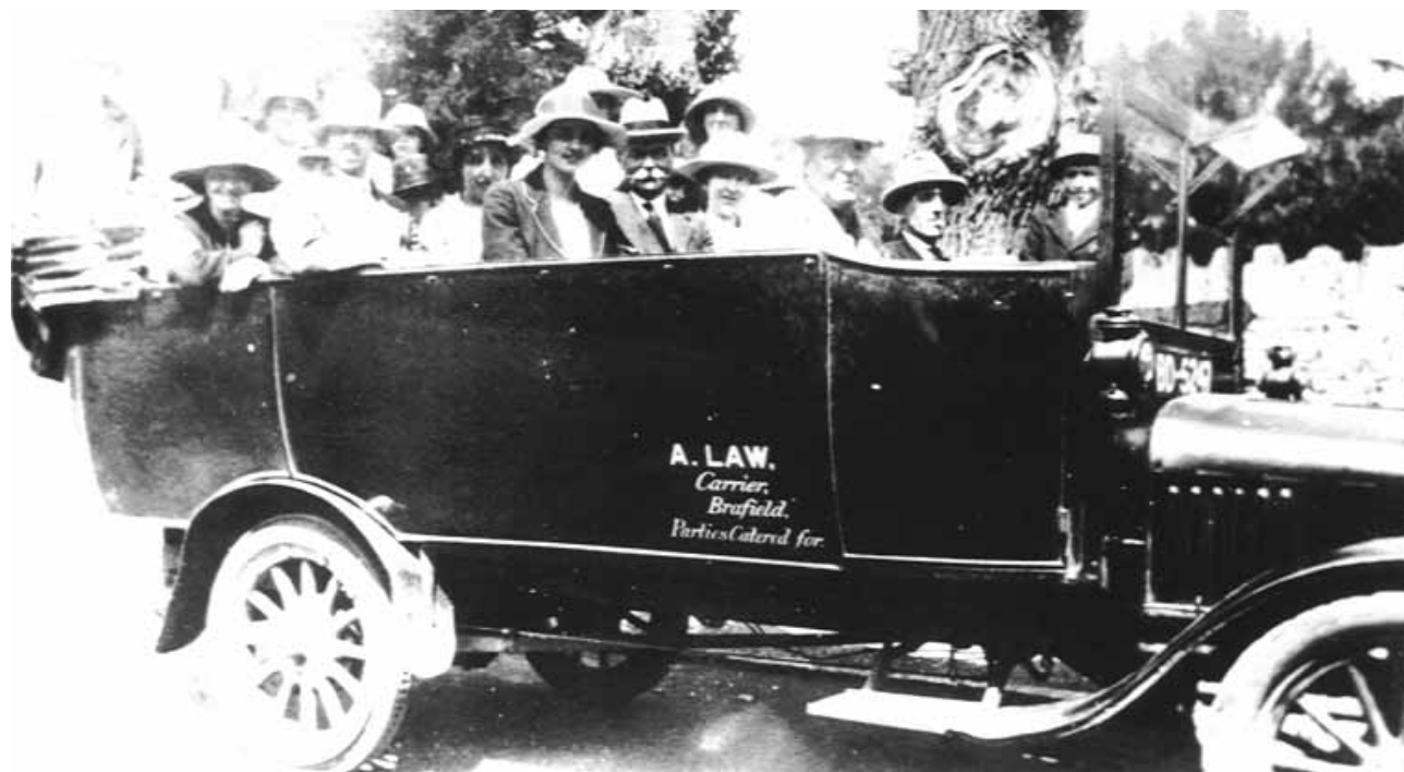
Andrew Law's first motorised passenger vehicle was this model T Ford registered BD 5247 in January 1921 and bodied by Ben Hasker of Northampton.
