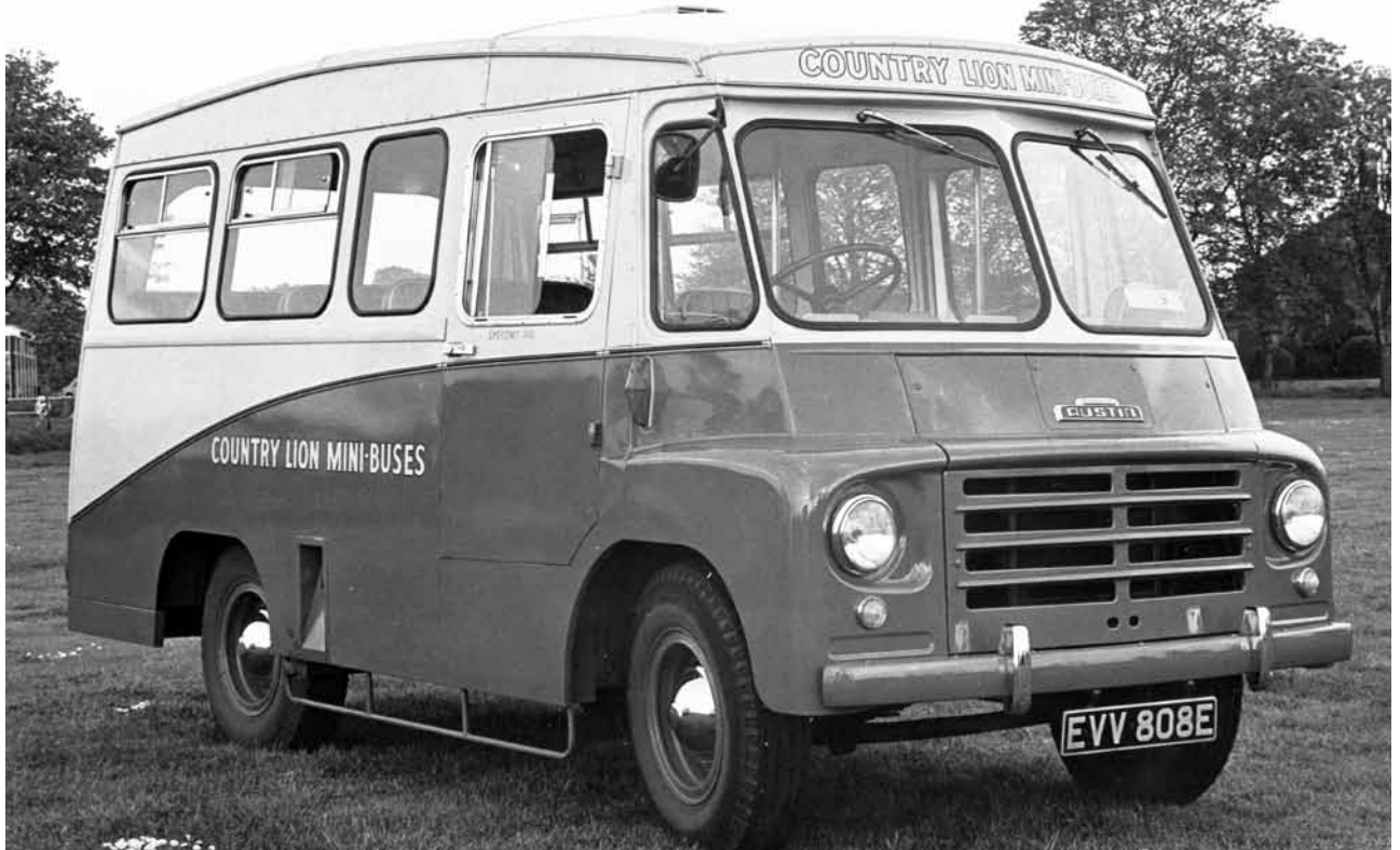
These BMC vans made quite attractive minibuses as is shown by EVV 808E, an Austin/Martin Walter fourteen seater.
