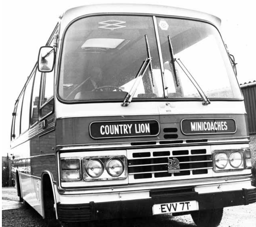
EVV 7T was one of Country Lion's Duple Dominant bodied Bedford VAS5 twenty-nine seater coaches bought new in 1979 and it was retained for four years.
