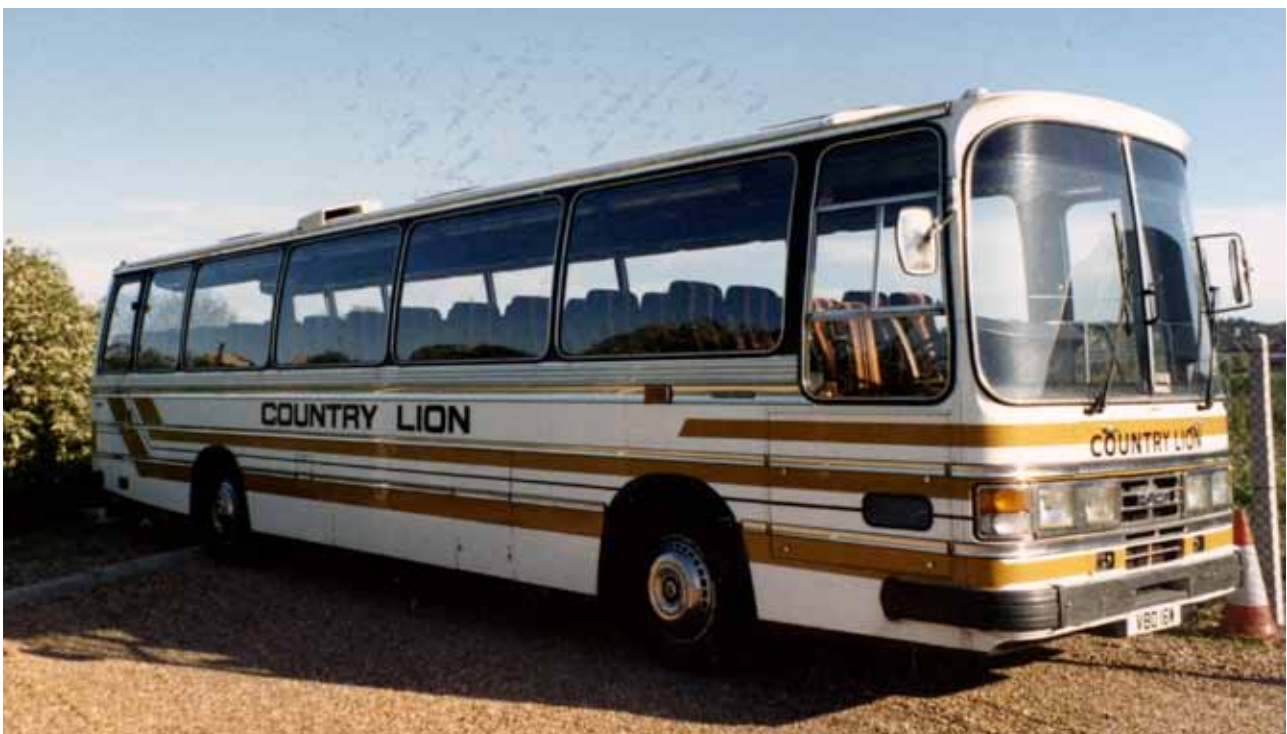
Duple built a Dominant coach body for fitment to this Ford R1114 chassis which was delivered to Palmerston Garage as VBD 16W.
