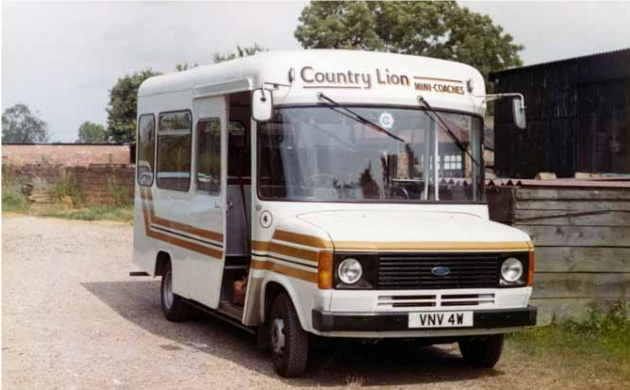
VNV 4W, a 1981 Ford Transit/Dormobile sixteen seater looks immaculate as it stands in the sun.
