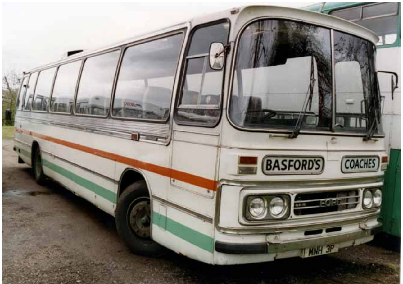
One of the two Ford coaches taken over with Basford's was MNH 3P which dated from 1976 and carried a Duple Dominant body accommodating fifty-three passengers.
