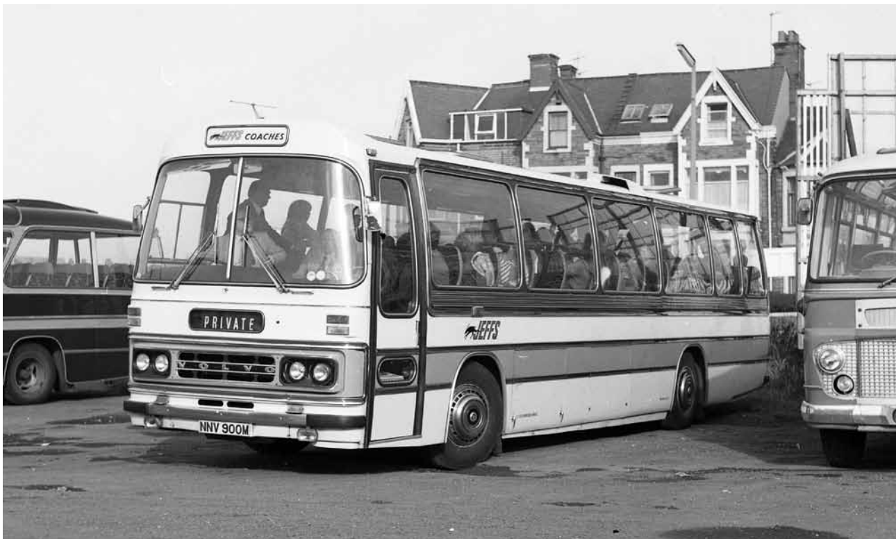
A nearside view of Jeffs' Volvo B58 registered NNV 900M with its Duple Dominant coachwork, operating one of the many school private hire trips undertaken by Jeffs' Coaches. (Photo courtesy R Marshall).
