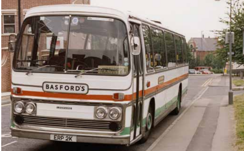
ERP 2K was a 1972 Leyland Leopard with a fifty-one seat Plaxton Elite Express II body. It was photographed in Victoria Street, Northampton when twenty years old.
