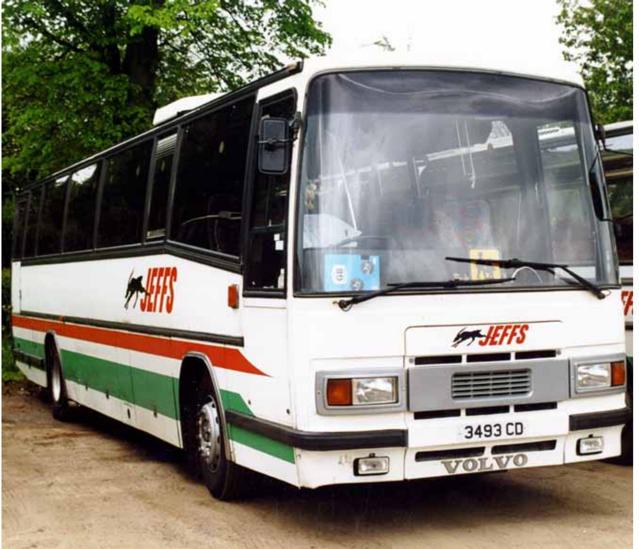
3493 CD a Plaxton Paramount 3200-II bodied Volvo B10M-61 was eight years old when it entered the Jeffs' Coaches fleet from Dore International.
