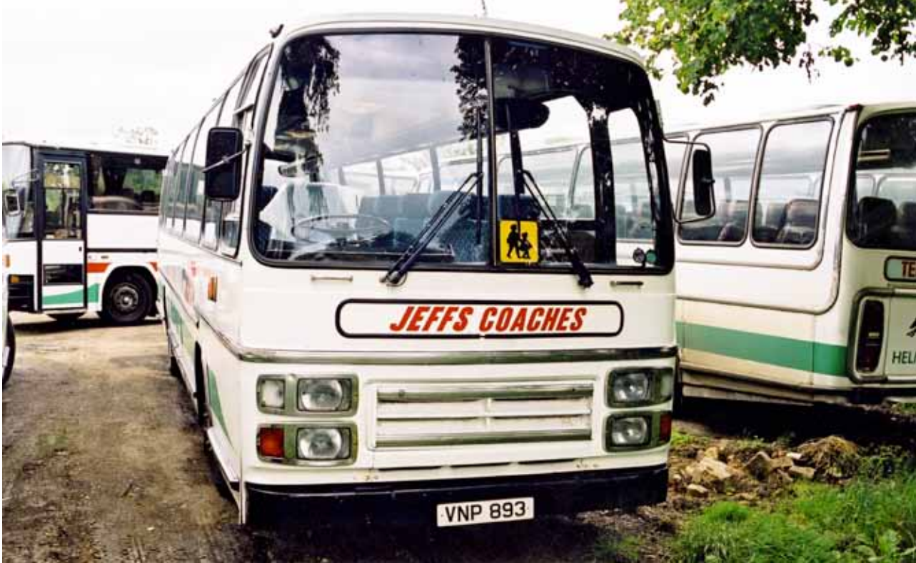
Unlike YFC 16/7V with Duple bodies, VNP 893 was fitted with Plaxton Supreme IV coachwork as can be seen in this view of the Leyland Leopard.
