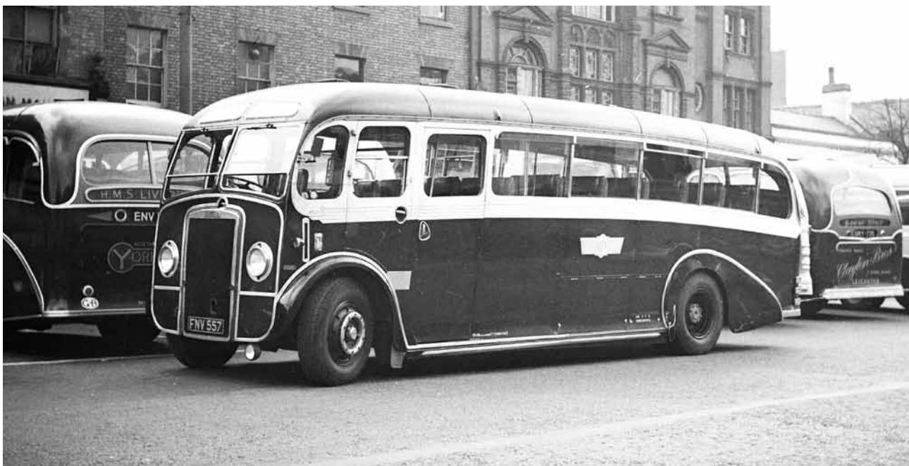
This distinctive Leyland Tiger coach carried a body built by Whitson to a fully-fronted design. FNV 557 seated thirty-three passengers and has since been preserved, albeit not painted in the livery in which it was adorned whilst with Royal Blue. The location for this photograph was Humberstone Gate, Leicester. (Photo courtesy R Marshall)
