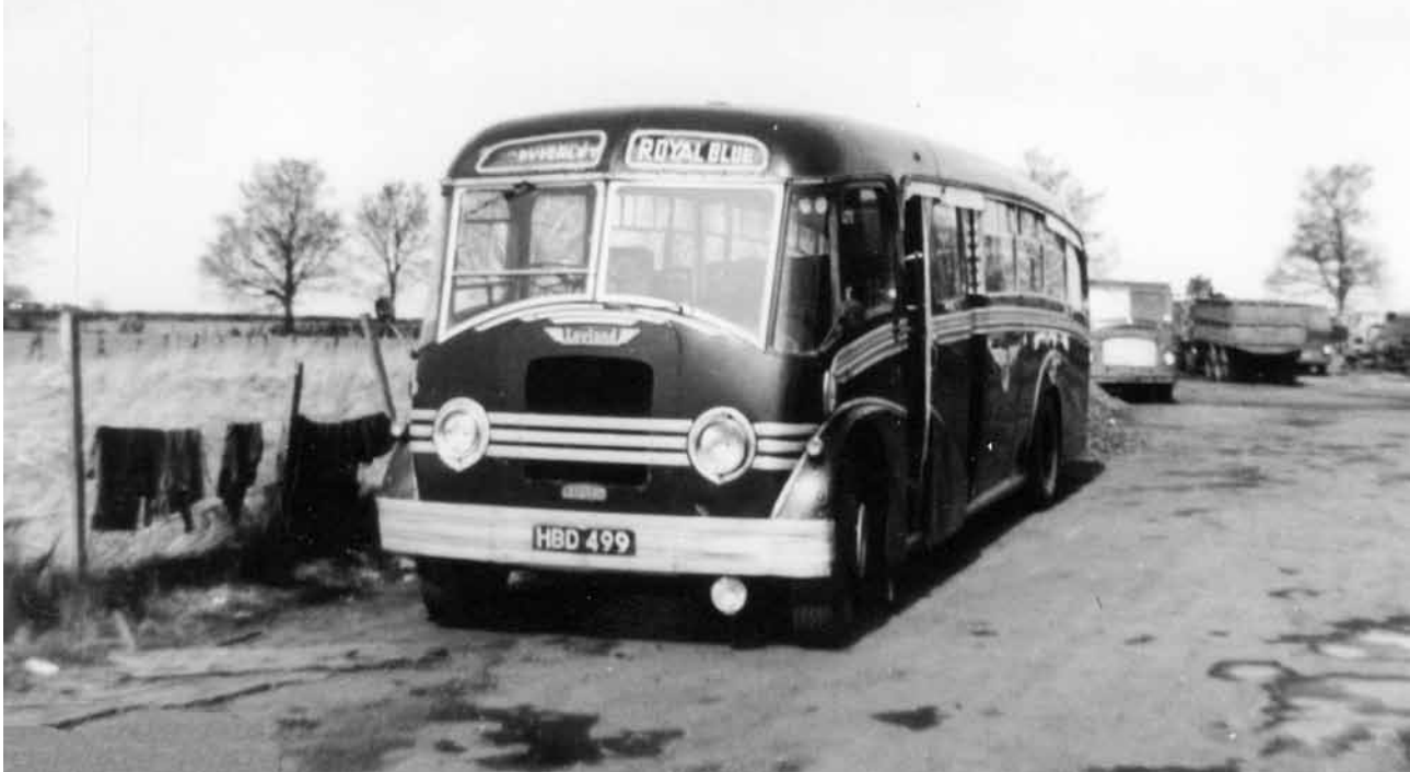
In contrast to GNV 999, the March 1952 delivery of a Yeates bodied Leyland Tiger PS2 in the shape of HBD 499, with its enormous fender and excessive chrome decorative strips gave this coach a somewhat ungainly appearance. The picture was taken at Church's Pytchley garage. (Photo courtesy T Roberts)
