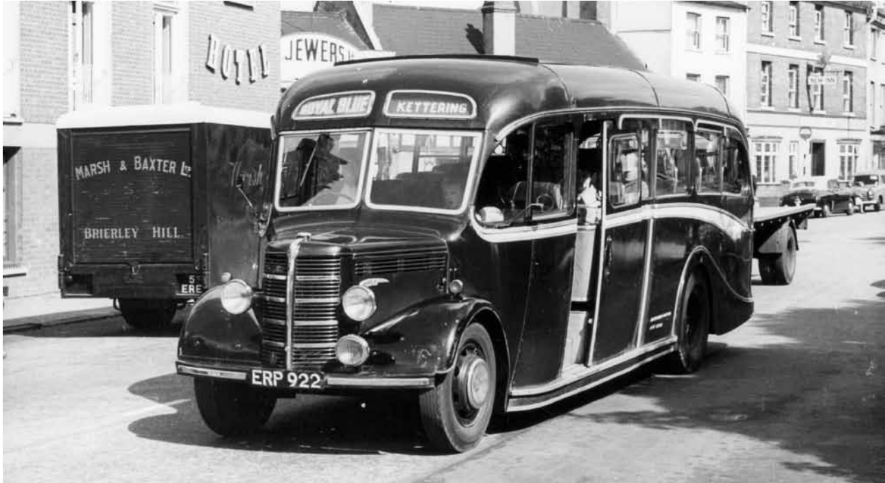
The first new bus delivered after the War was ERP 922, a Bedford OB with standard Duple Vista 29-seat bodywork. During the seventeen years Royal Blue owned this vehicle it was a regular performer on the stage-carriage services and proved a most reliable machine. This picture was taken at Kettering Library. (Photo courtesy R H G Simpson)
