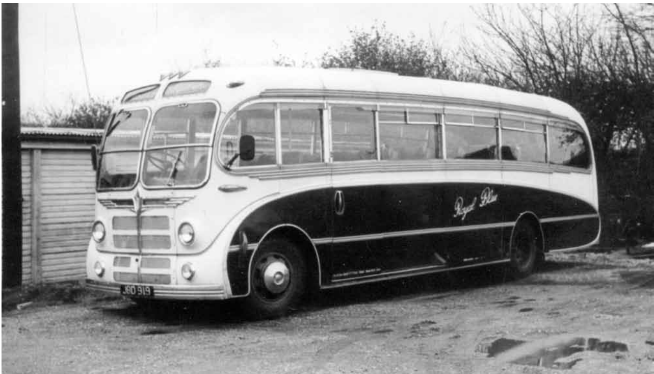
The timeless design of the Burlingham Seagull body is apparent in this view of Royal Blue's Bedford SBG registered JBD 919. (Photo courtesy T Roberts)
