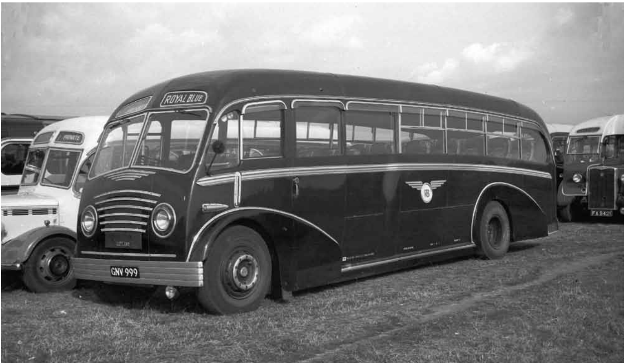
GNV 999 was a Leyland Tiger PS2 fitted with a rather pleasant fully-fronted Yeates coach body seating thirty-five passengers. It was new to Royal Blue in April 1951.
