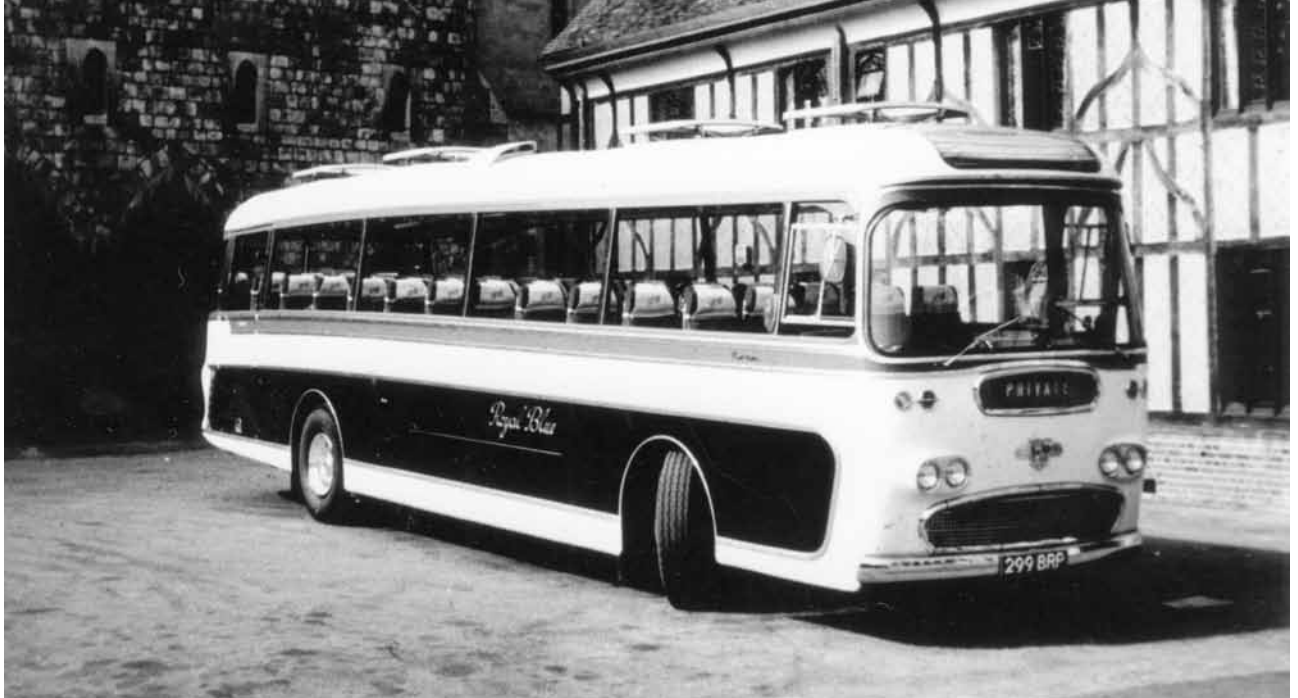
299 BRP was a fifty-one seater Plaxton Panorama bodied Leyland Leopard which dated from 1962. It was parked in the courtyard of Windsor Castle when it was photographed.
