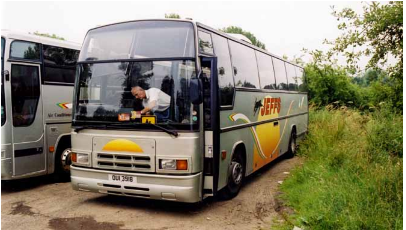
The high floor Plaxton Paramount 3500 bodied Volvo B10M incoming to Jeffs' from York Brothers was OUI 3918. With Bowen's having a standard livery only the company name and logo transfers needed changing.
