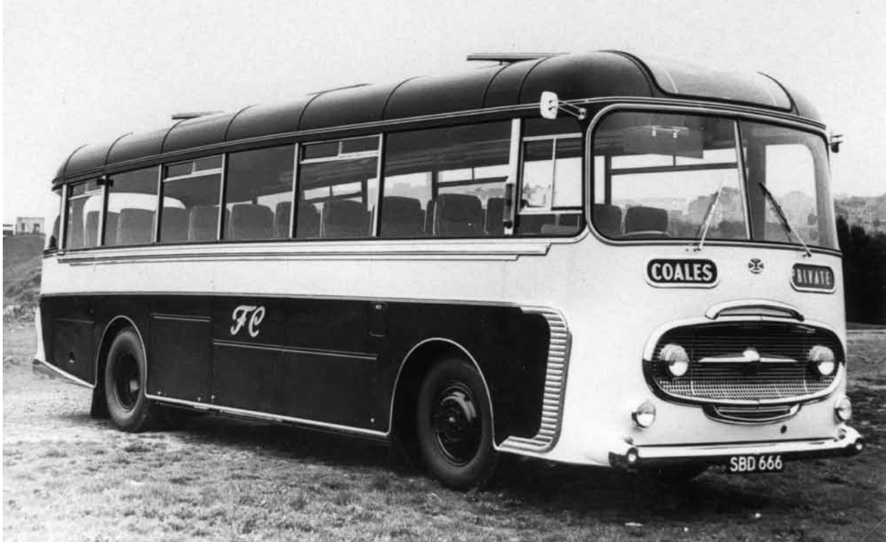
Coales' final new coach was SBD 666, a Plaxton Consort bodied Albion Aberdonian of 1958 vintage which entered service in January 1959. This view shows the front offside of SBD666. (Photo courtesy Plaxton's)
