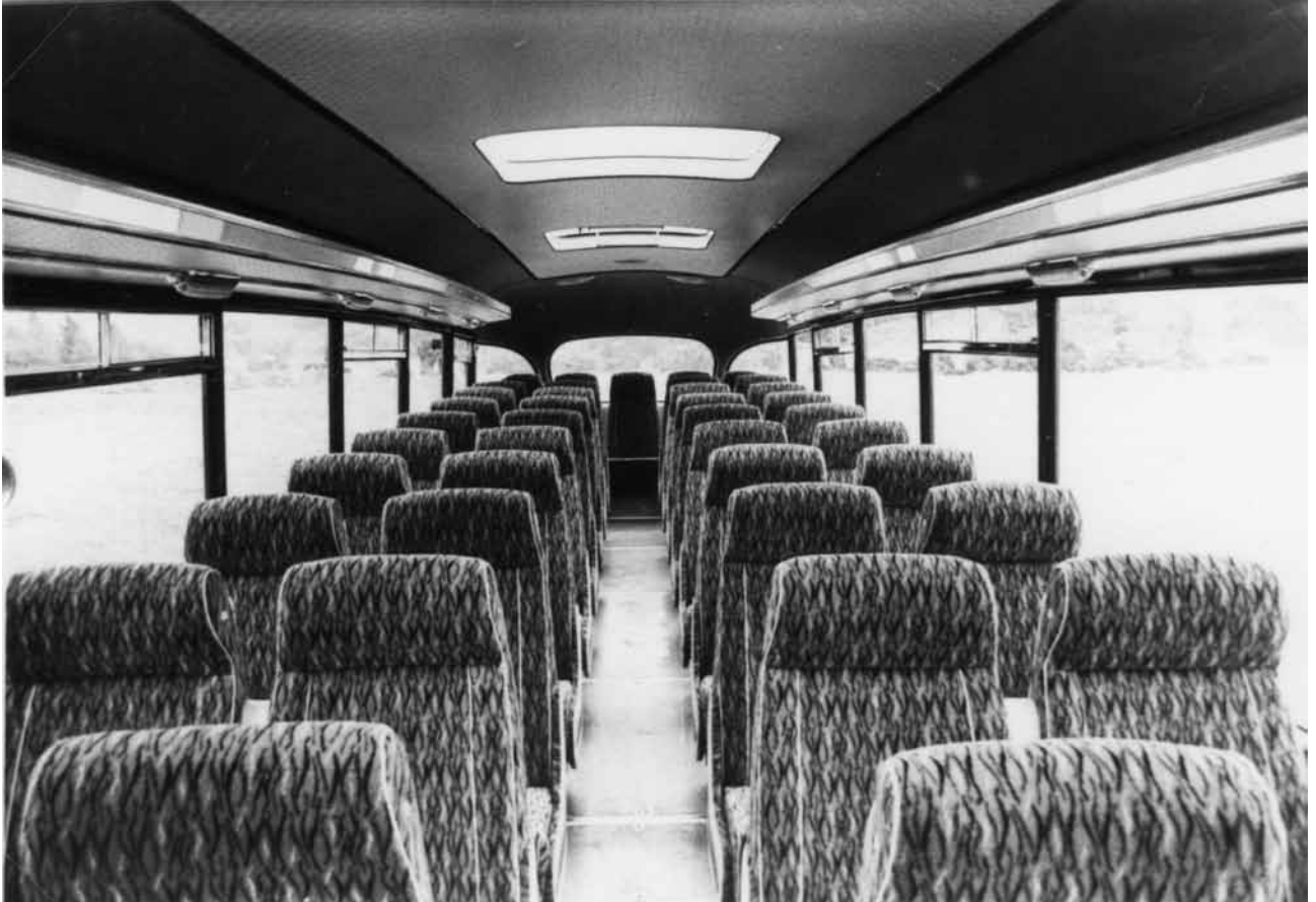
An interior view of the Plaxton Consort body carried by SBD 666. (Photo courtesy Plaxton's)
