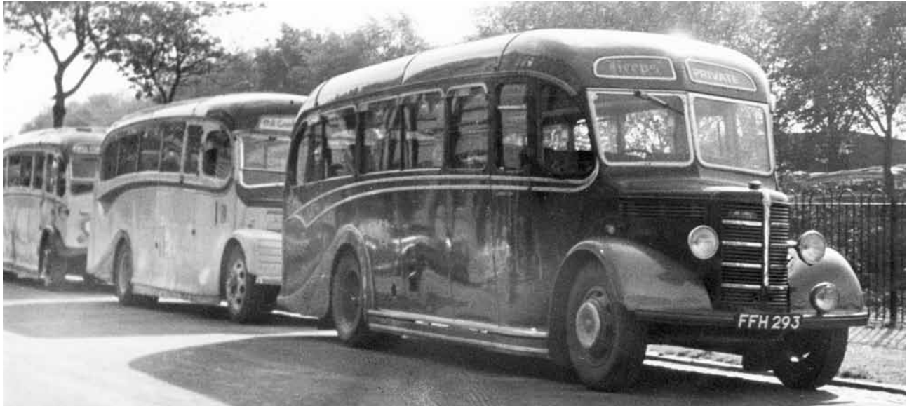
FFH 293 was a standard Duple Vista bodied Bedford OB which provided several years of good service to Peter Chapman prior to being sold for non-P.S.V. use to the associated building firm of Lucas of Moulton. (Photo courtesy D M Bailey).
