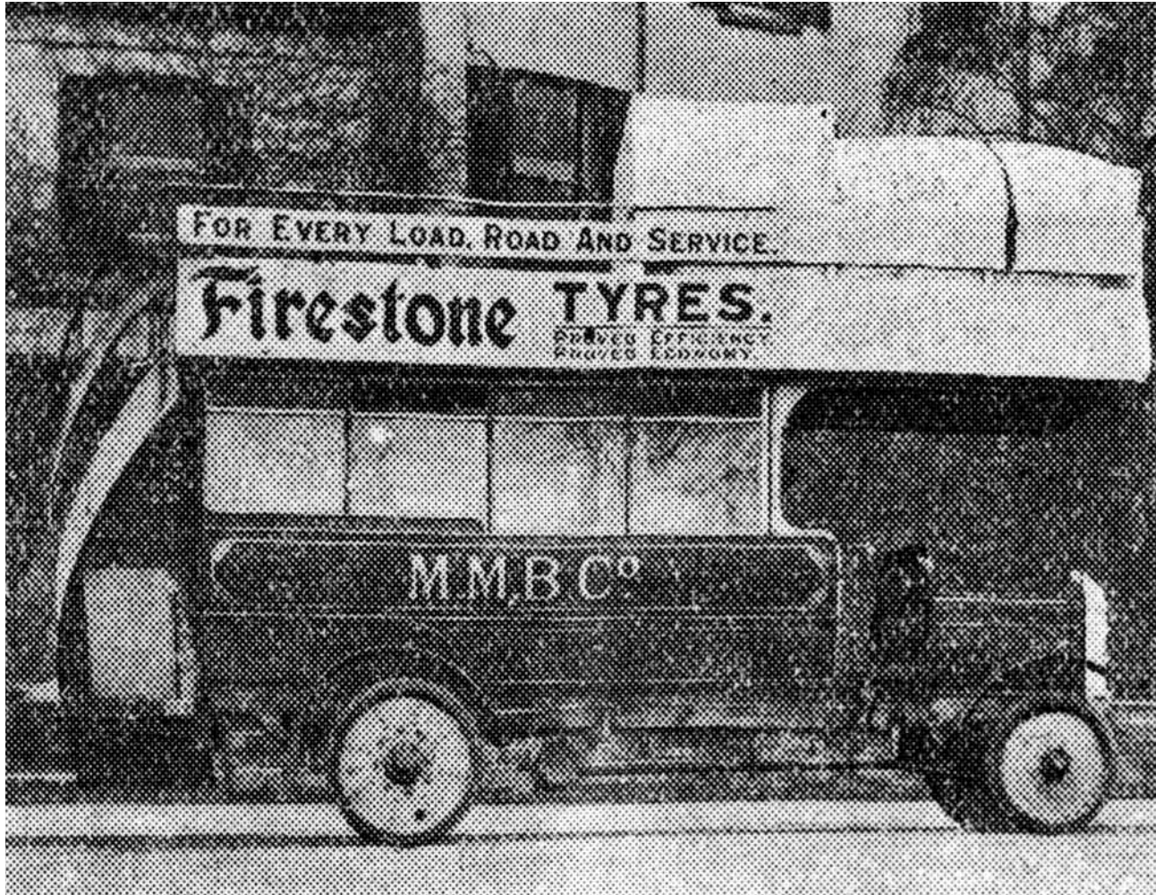
One of the M.M.B.Co's Straker-Squire double decks operating on town gas in 1917. Note the forward position of the gas bag and extended superstructure of the bus. It was said that one bag of gas was equal to 1½ gallons of petrol and at a quarter of the cost.
