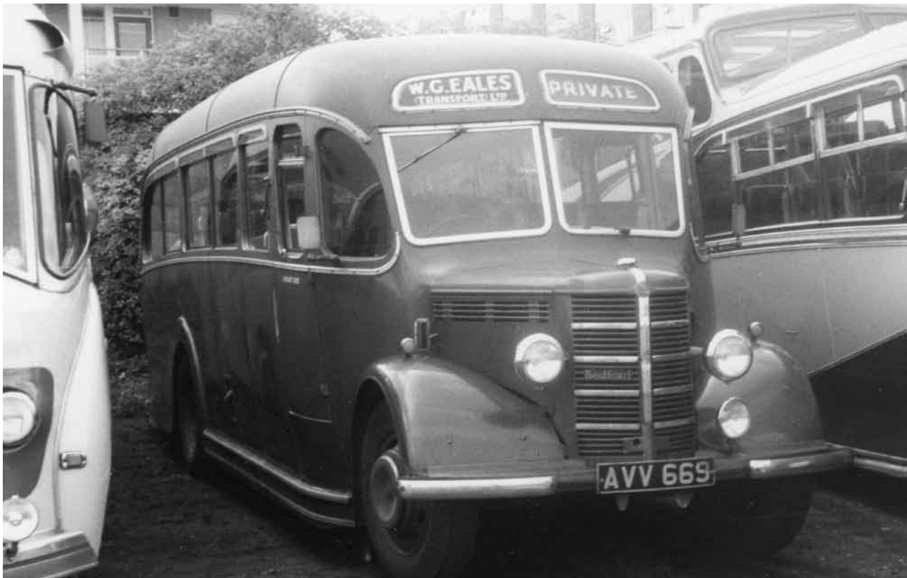
This photograph, taken in September 1962, shows W G Eales' Bedford OB coach AVV 669 with its twenty-nine seat Duplex V body. As will be seen, its coachwork was kept in pristine condition. (Photo courtesy F Gainsbury)
